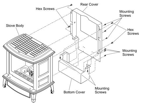
Figure 16 - Removing Rear Cover and Bottom Cover from Stove Body
